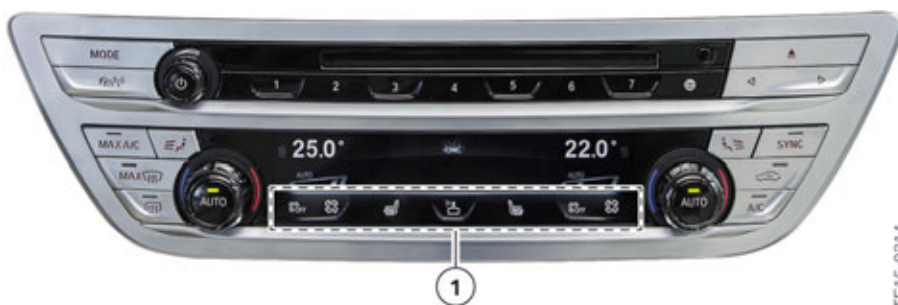
G12 4-zone IHKA control panel with touch operation
